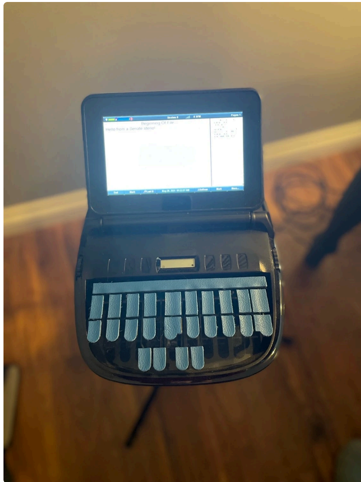
A stenography machine with the words "Hello from a Senate steno" in English and steno displayed on screen.
